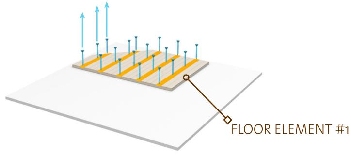
ATTACH FLOOR ELEMENTS ASKERSUND 40 WITH SCREWS. Ø 5 mm
