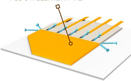
SLIDE THE MIDDLE FLOORBOARD BACK IN AND RE-ATTACH IT WITH SCREWS. 2%
